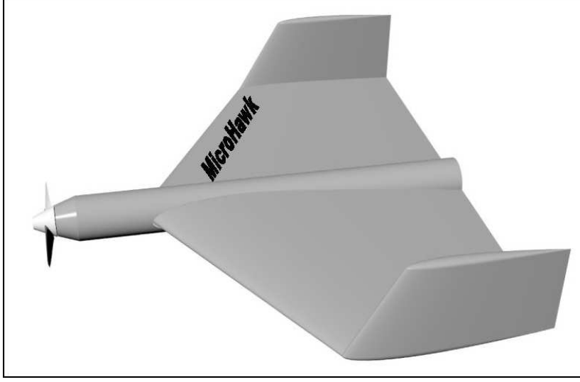
Figure 2. The micro aerial vehicle configuration (MicroHawk).
