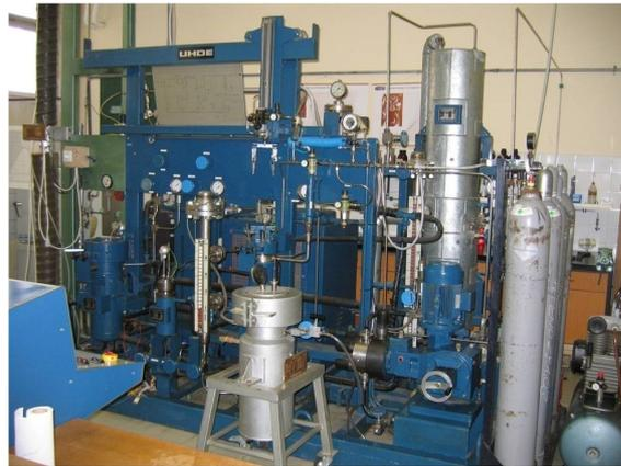
Figure 2. High pressure extraction unit (Faculty of Chemistry and Chemical Engineering, University of Maribor, Slovenia).
