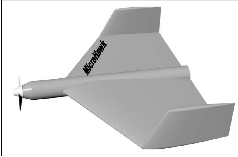
Figure 2. The micro aerial vehicle configuration (MicroHawk).
